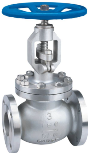
Globe Valve 3" #150 SS ASTM A351 CF8
